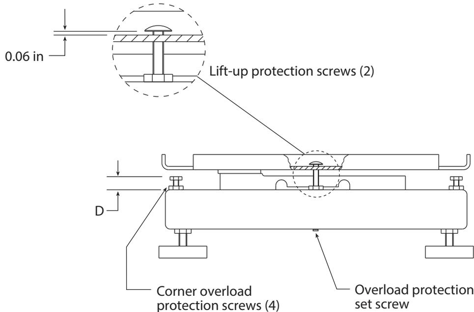
Figure 2-5. RL2100 Protection Screw Adjustments
