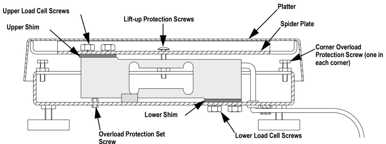
Figure 2-4. RL2100 Components – Side View
