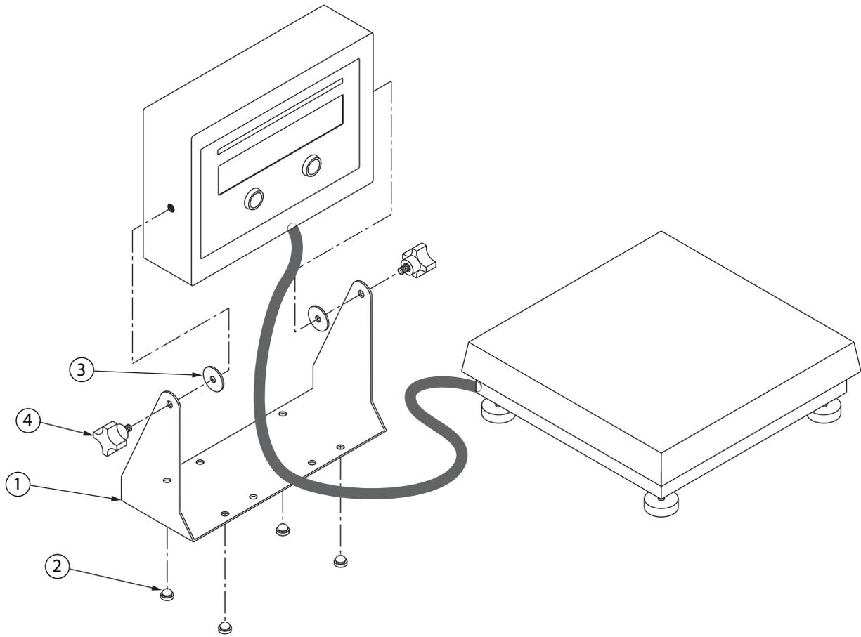
Figure 2-9. IQ Plus 210 Tilt Stand Assembly
