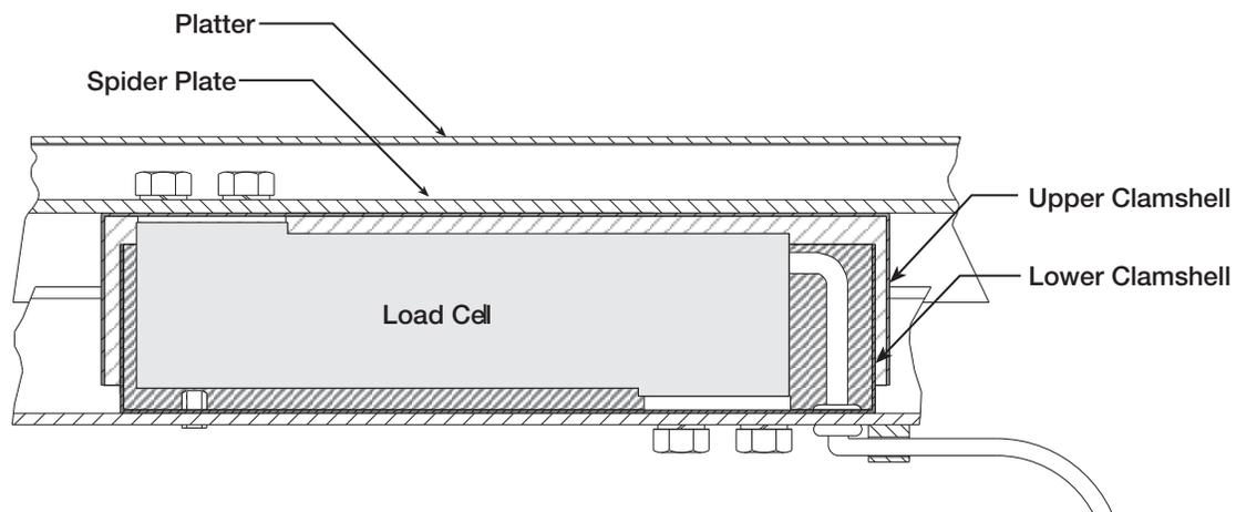
Figure 2-6. Clamshell Installation
