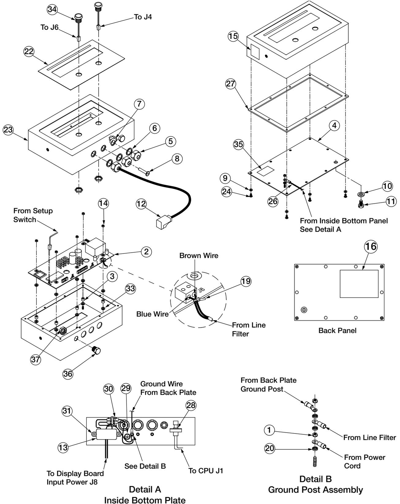
Figure 2-7. IQ Plus 210 Indicator Parts Illustration
