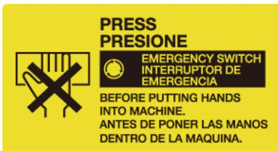
In case you have to put your hand in the machine during operation or in case you hear strange noises from the machine, or when there is a possibility that can cause a dangerous situation if you leave the machine on, please press the EMERGENCY SWITCH, and then continue the maintenance operation.
