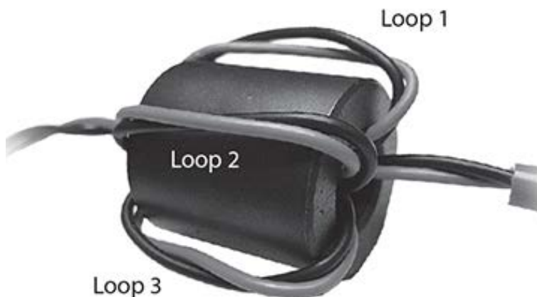
Figure 2-5. Cylindrical Ferrite Placement for RF Interference
