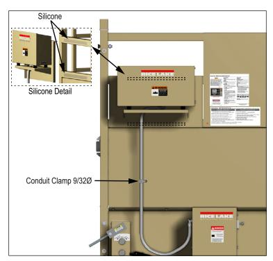
Figure 2-6. Weighcenter Mounting
