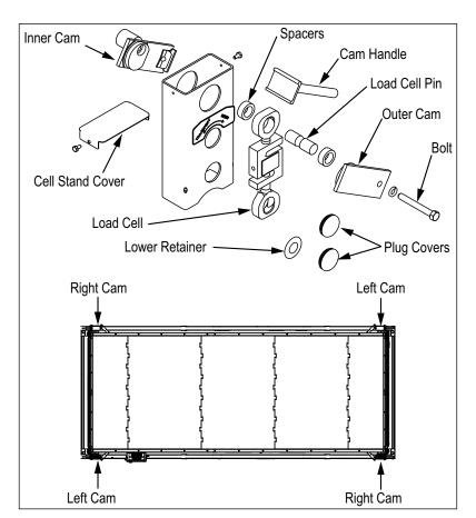
Figure 5-2. Disassembly and Greasing
