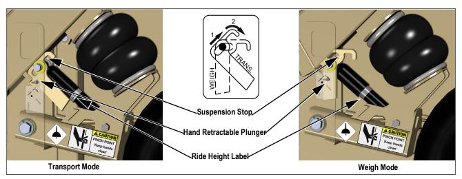
Figure 3-2. Suspension Stop and Ride Height
