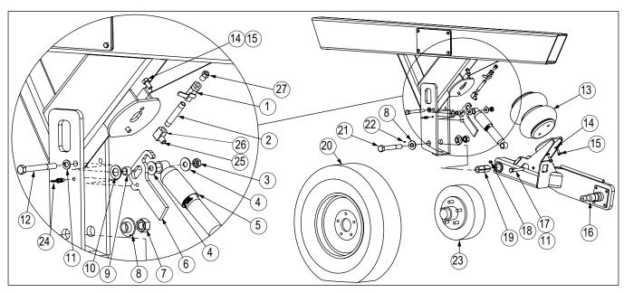
Figure 4-4. Tire/Wheel Parts
