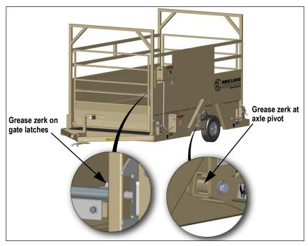
Figure 5-1. Grease Zerk Locations
