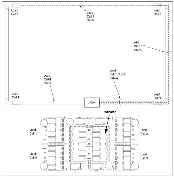
Figure 2-10. Load Cell Wiring Diagram
