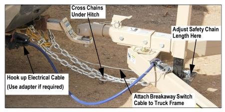
Figure 3-1. Hitch Connection
