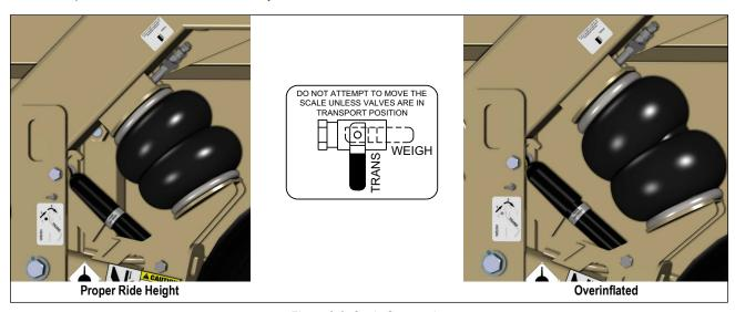
Figure 3-6. Scale Suspension
