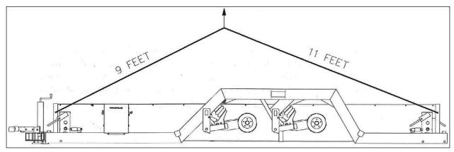
Figure 1-5. Slinging the Scale
