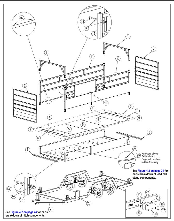
Figure 4-1. MAS-M Scale Parts Illustration
