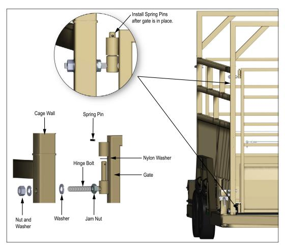
Figure 2-3. Assemble Gate to Scale
