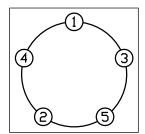
Figure 2-1. Wheel Torque Pattern
