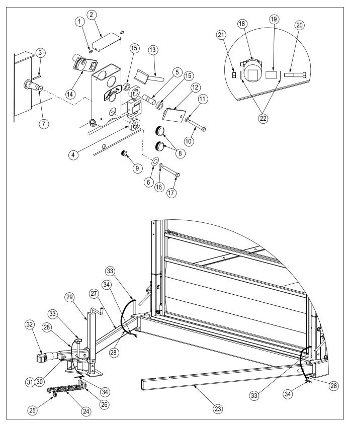
Figure 4-2. Hitch and Load Cell Stand Component Details
