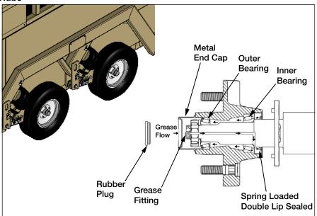
Figure 5-3. Hub Lubrication
