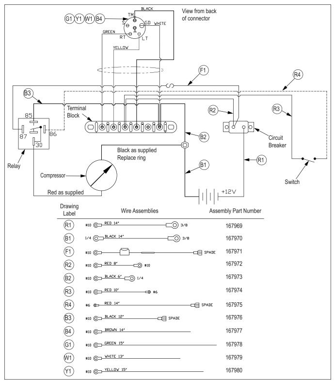
Figure 4-6. Battery Box Wiring Parts Illustration
