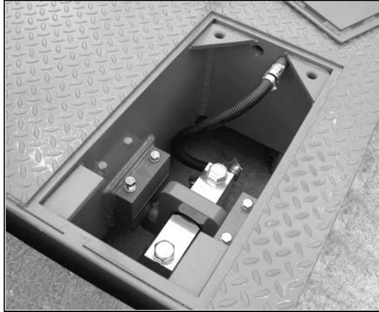
*Figure 4-4. Top View of Load Cell Access Arena*
