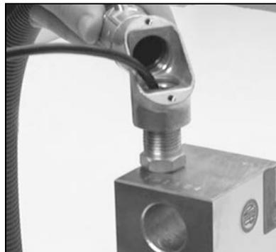
Figure 4-3. Installing 90° Fitting to Load Cell
