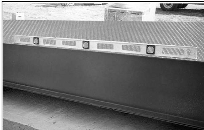
Figure 3-8. Check Weighbridge for Level
