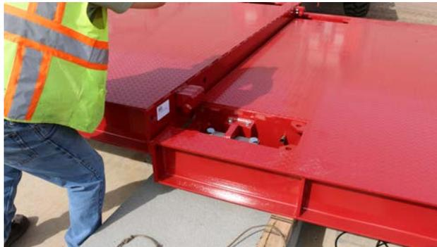
Figure 3-6. Pin and Receptacle Interface
