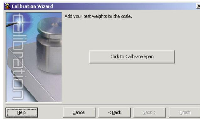
Figure 12. *iRev Span Calibration Display*
