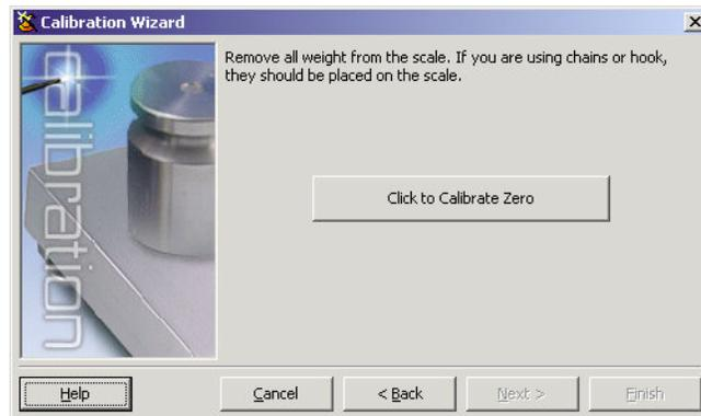
Figure 11. iRev Zero Calibration Display
