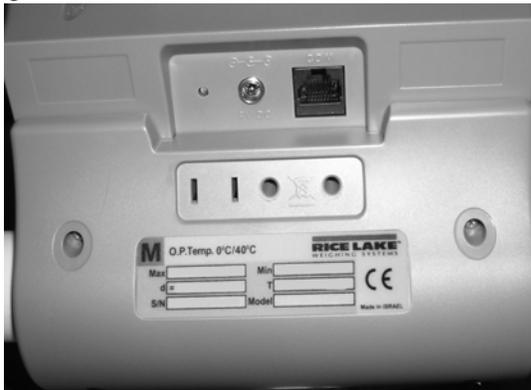
Remove retaining screws x 4 (only 2 shown)
