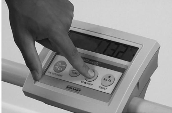
*Figure 2-9. Press The Reweigh Key to Verify Weight*
