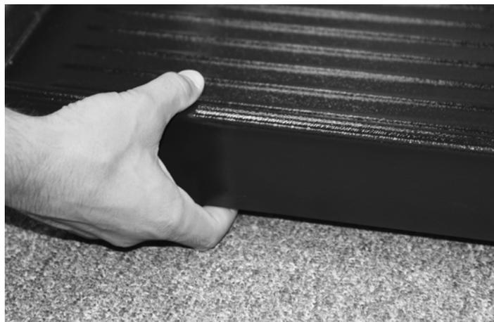
Figure 2-5. Have a Minimal Amount of Clearance Between the Scale Base and the Floor
