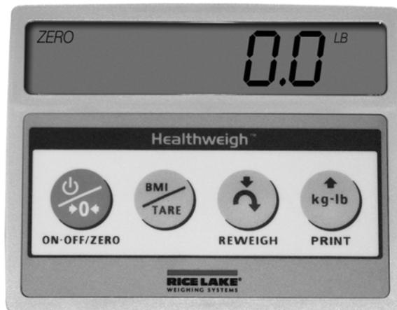
Figure 3-1. Front Panel Display Keys
