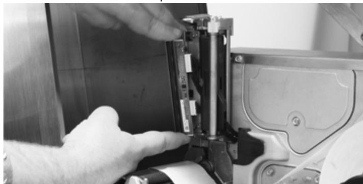
Figure 3-2. Remove Old Printhead Assembly
