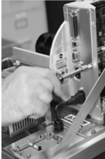
Figure 5-21. Remove Screws from Cover Plate
