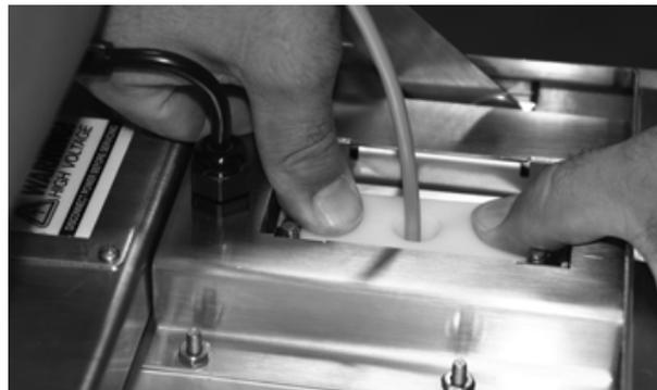
*Figure 1-12. Seat the Split Seal Assembly*
