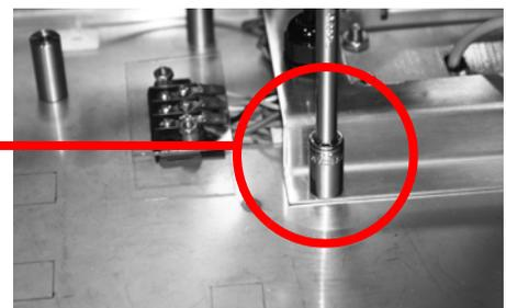
Figure 5-10. Secure Heater to Enclosure Bottom
