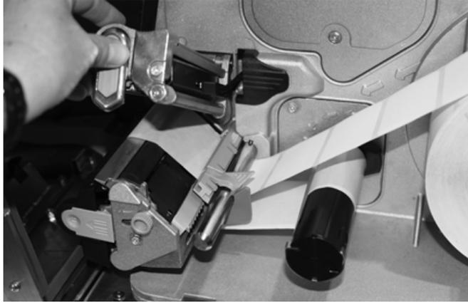
Figure 1-30. Flip Mechanisms Back Down to Secure Labels
