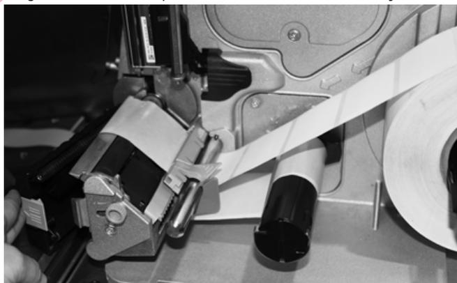
Figure 1-29. Place Backing Material onto Internal Rewinder
