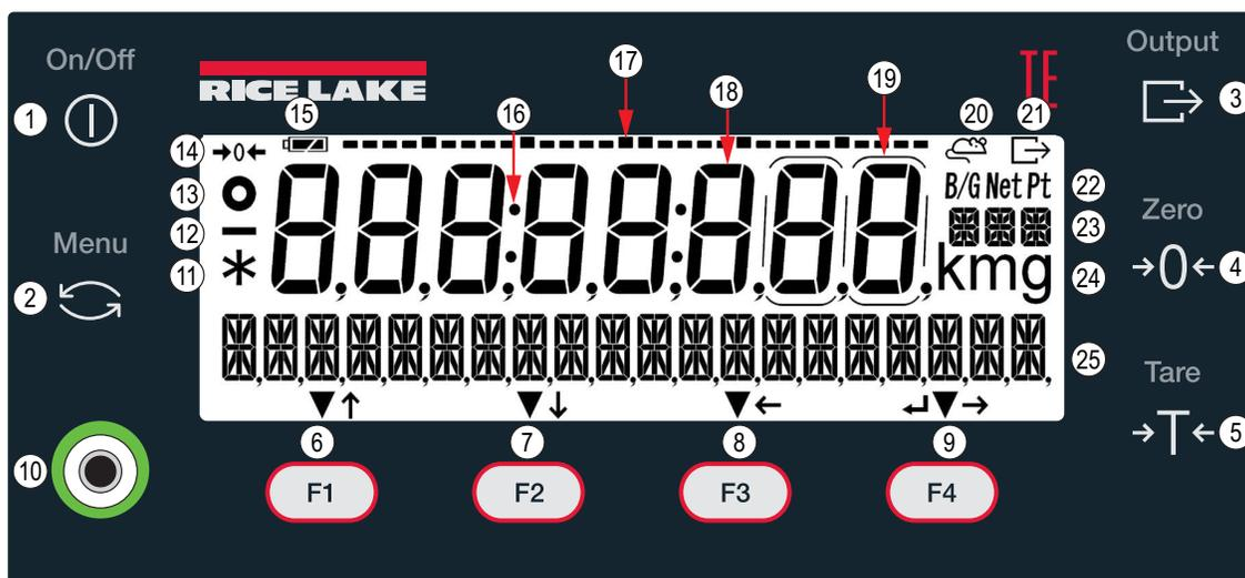
Figure 3-1. Front Panel Display Overview (NTEP Only Models)
