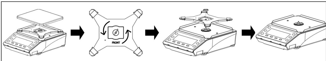
Figure 7-2. Disassemble to Clean
