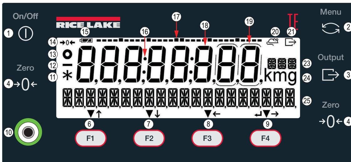
Figure 3-2. Front Panel Display Overview (NTEP/Measurement Canada Models)
