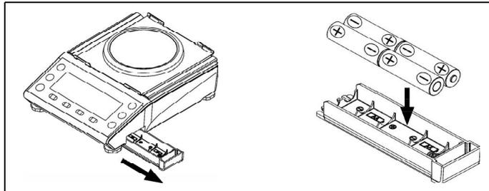
Figure 2-5. Install Batteries
