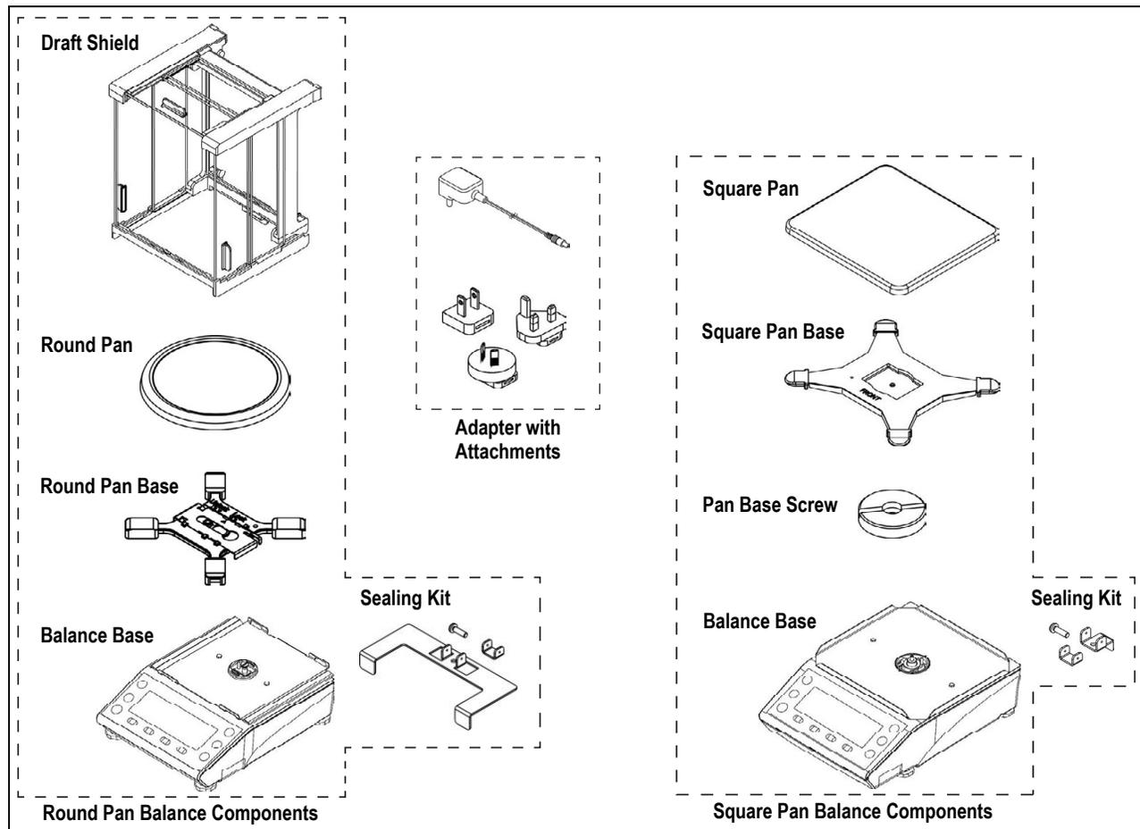
Figure 2-1. Balance Components
