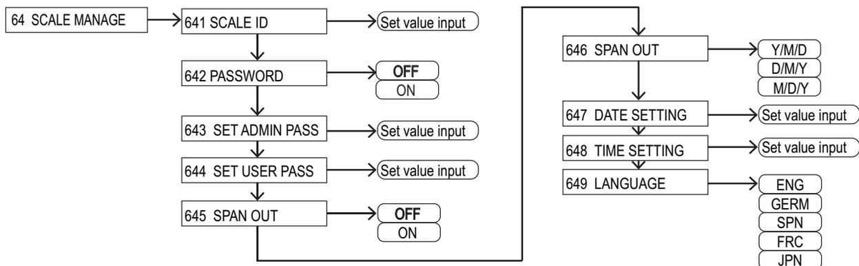
Figure 4-10. Controlling and Adjusting–Balance Manage Menu Layout
