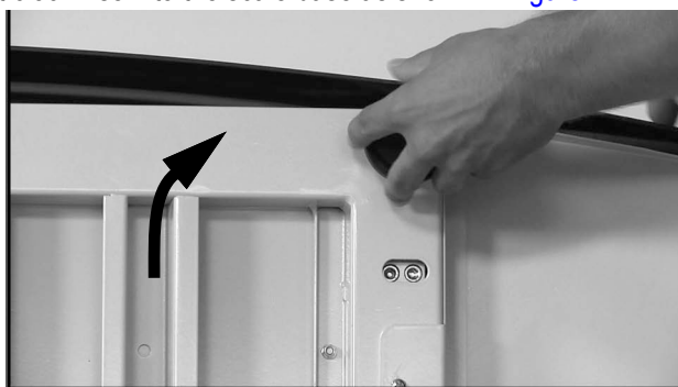
Figure 2-1. Screw Feet Into the Scale Platform
