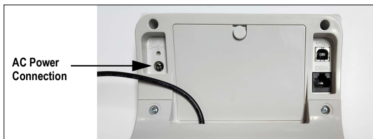
Figure 2-8. Power Connection Site
