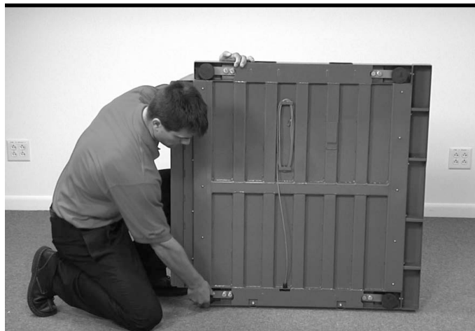
Figure 2-3. Backing out the Scale Feet
