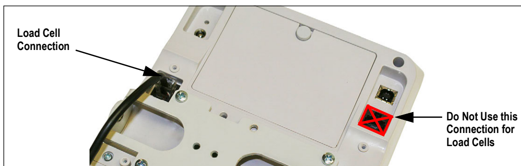
Figure 2-8. Load Cell Connection Point
