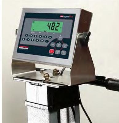
Figure 4-6. Secure Indicator to Base Plate
