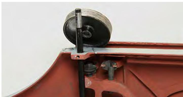
Figure 2-3. Place Washers and Wheels on Each Axle
