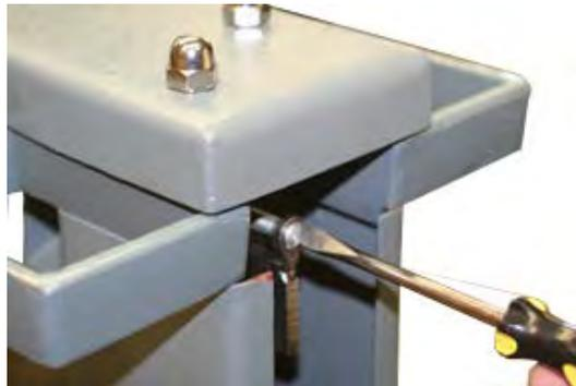
Figure 2-18. Zero Adjustment Location
