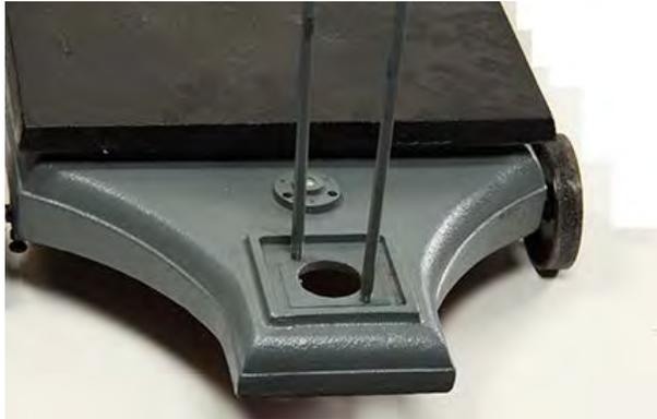
Figure 2-7. Screw Pillar Rods into Scale Platform
