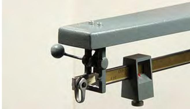
Figure 2-16. Secure Trig Loop Assembly with Bolts
