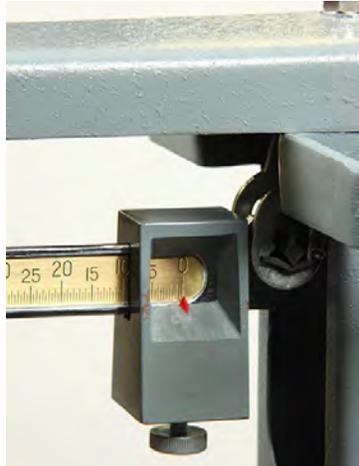
Figure 2-19. Scale Reading on Zero
