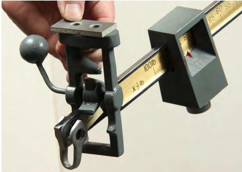
Figure 2-15. Inserting the Trig Loop Assembly to Beam Assembly and Adding the Trig Loop Mounting Plate
