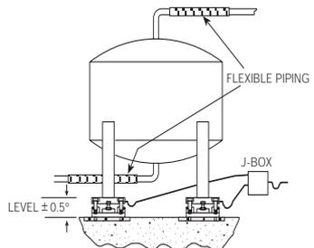
vessel to the first pipe support is 20 to 30 times the pipe diameter. In smaller, lower capacity tanks and hoppers, isolating the resultant forces becomes extremely critical. When possible, flexible conduit piping should be used close to the vessel instead of the rigid variety. For details, see our *Weigh Modules & Vessel Weighing Systems* manual, PN 43918.
