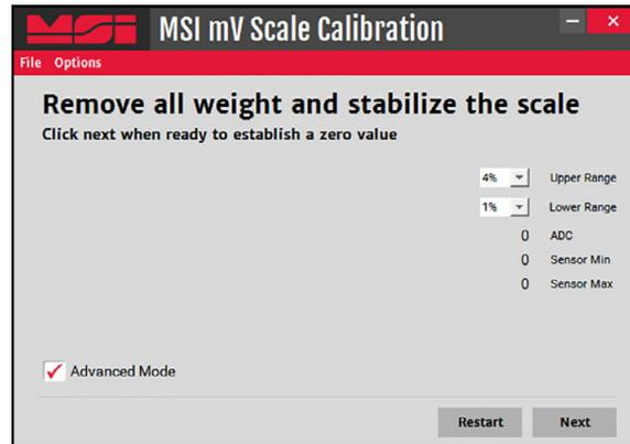
Figure 3-5. Zero Calibration
