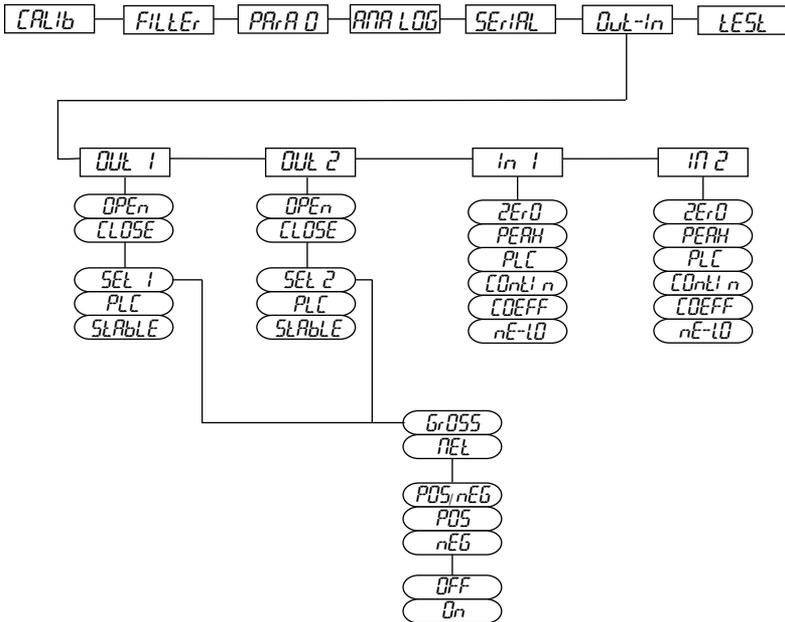
Figure 2-5. Outputs and Inputs Menu Structure
