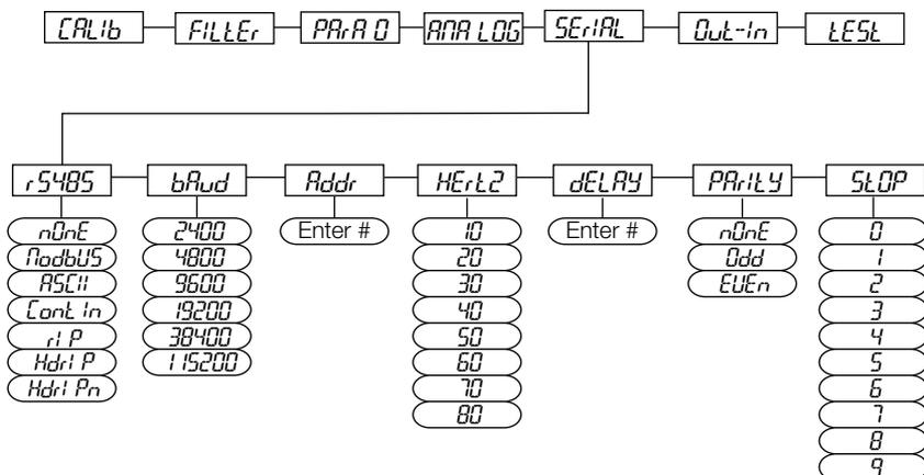
Figure 2-3. Serial Communications Menu Structure
