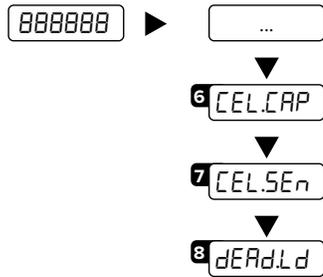
Set the total load cells capacity (up to 999999).
