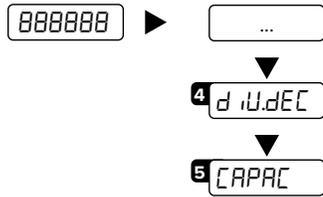
Set the decimal point position and the minimum scale increment\*<sup>1</sup>
