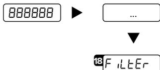
The active weight filter is displayed, alternating with the weight value.
