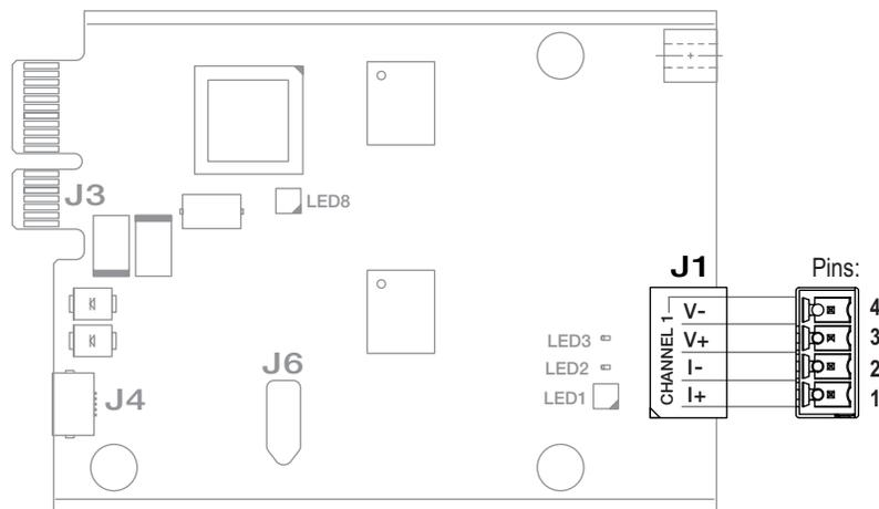
Figure 2. Analog Output Option Card
