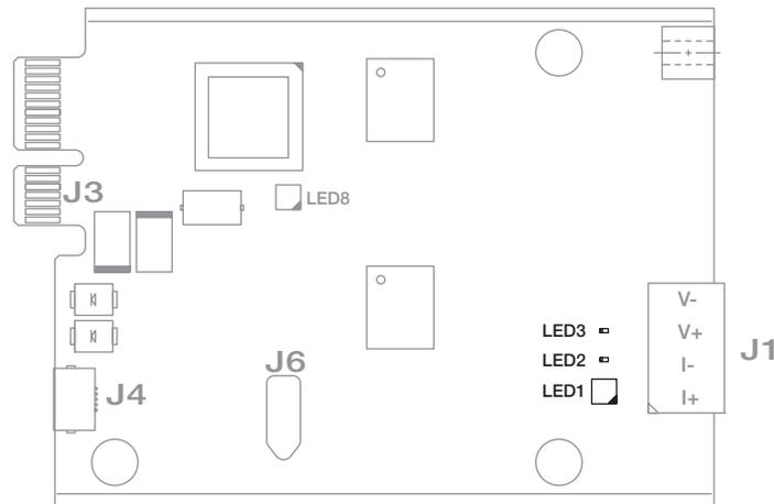
Figure 3. Analog Output Option Card LEDs
