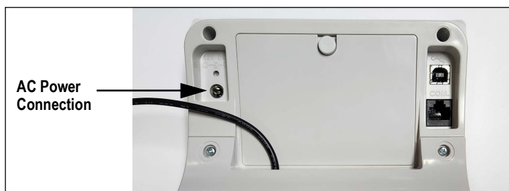
Figure 2-5. Power Connection Site
