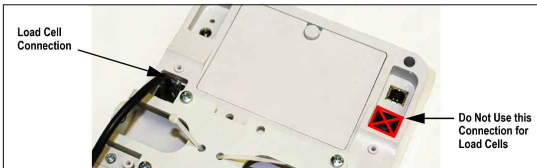
Figure 2-8. Load Cell Connection Point
