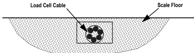
Figure 2-3. Cable Protection
