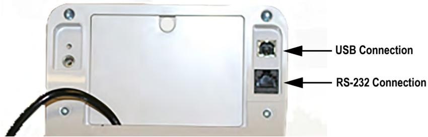
Figure 4-1. Connection Ports
