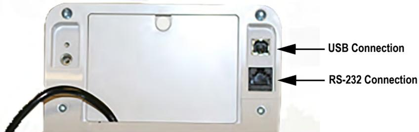
Figure 5-3. Connection Ports
