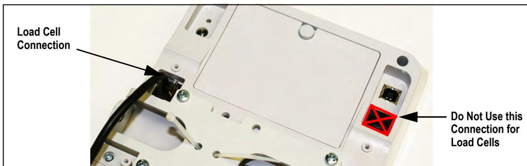
Figure 2-8. Load Cell Connection Point
