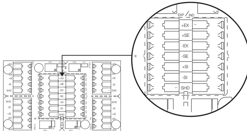
Figure 2-3. Expansion Port Wiring Location
