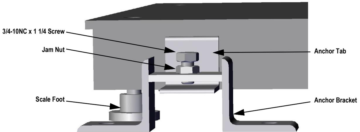
Figure 2-2. Anchor Bracket Installation
