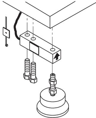
Figure 4-1. Load Cell Assembly
