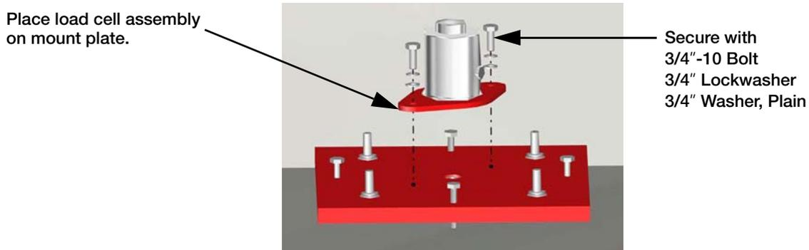
Figure 2-3. Load Cell Assembly to Mount Plate
