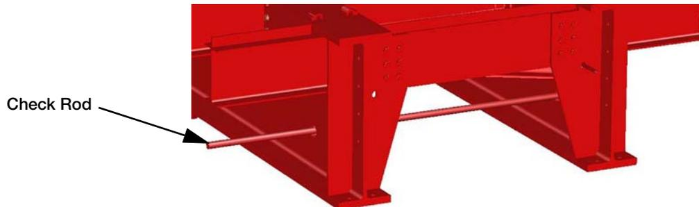
Figure 2-11. Check Rod Installation
