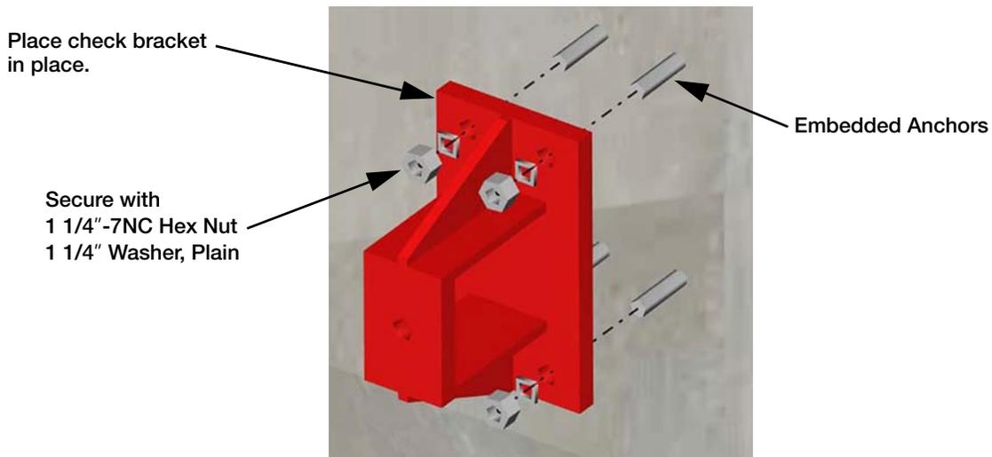
Figure 2-5. Check Rod Bracket on Foundation Side Wall
