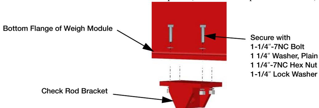
Figure 2-10. Check Rod Bracket on Weigh Module
