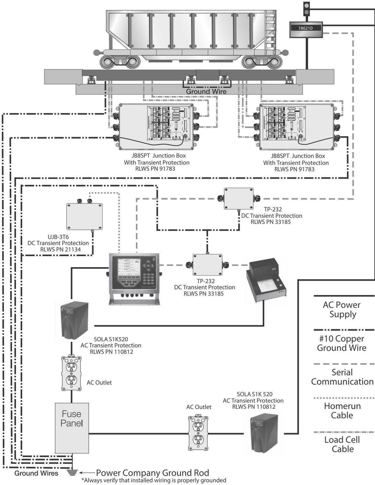
Figure 3-4. Single-Point Grounding Diagram
