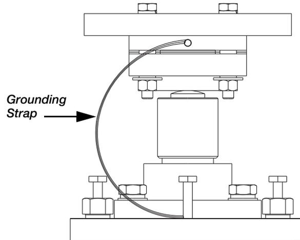
Figure 3-2. Grounding Strap on Load Cell Mount.
