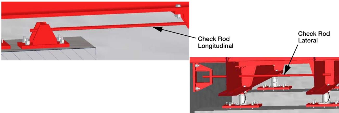
Figure 2-14. Check Rods to Foundation Check Rod Brackets
