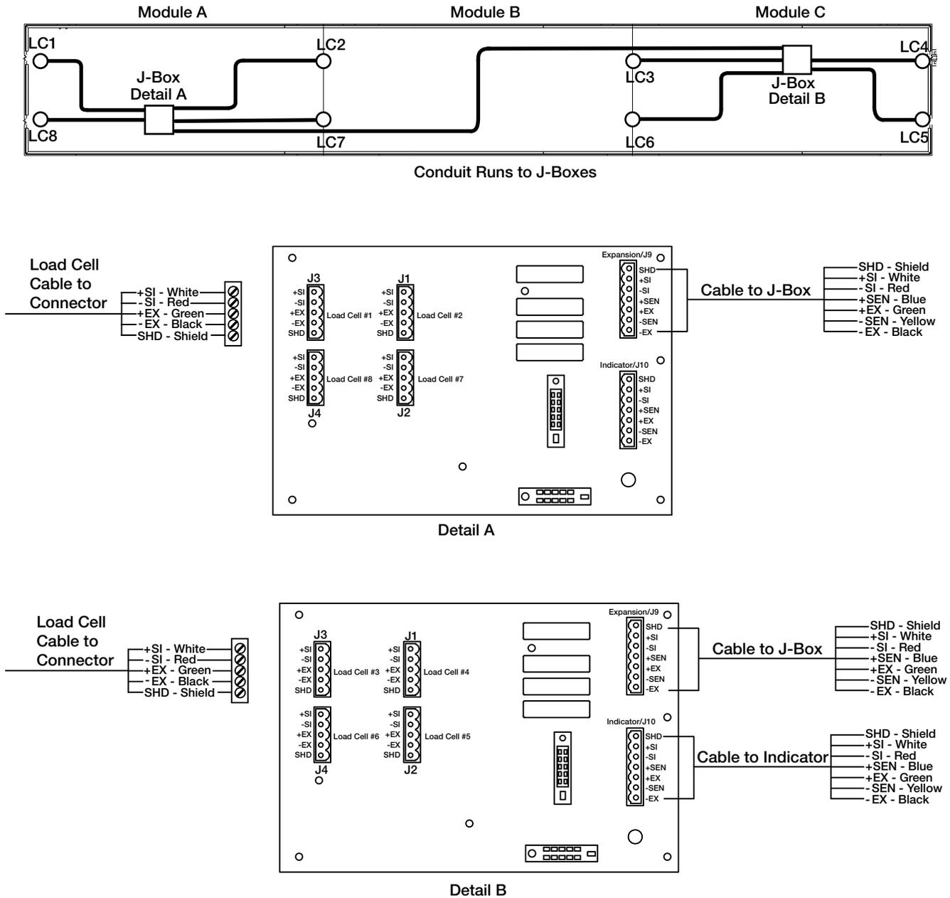
Figure 3-1. Junction Box Wiring and Conduit
