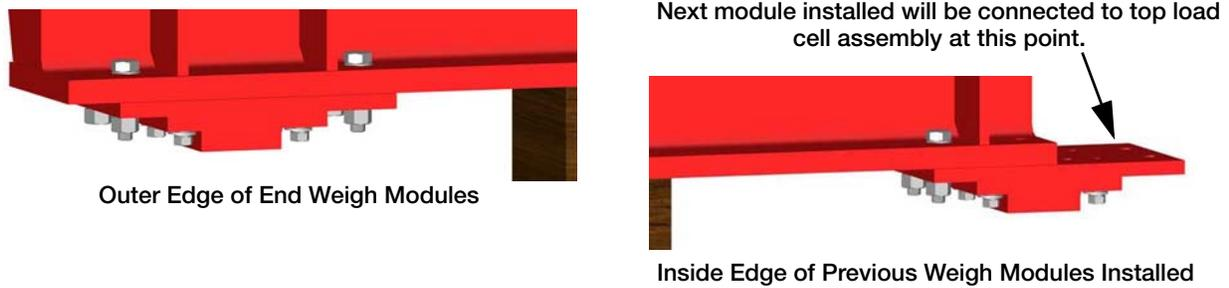
Figure 2-9. Top Load Cell Mount Assembly Placement
