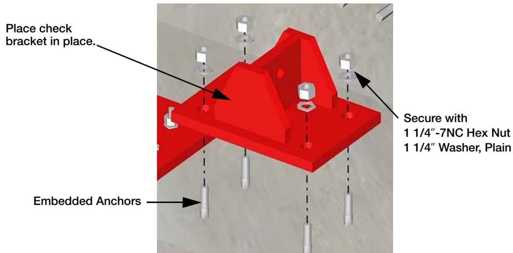
Figure 2-4. Check Rod Bracket on Foundation Base
