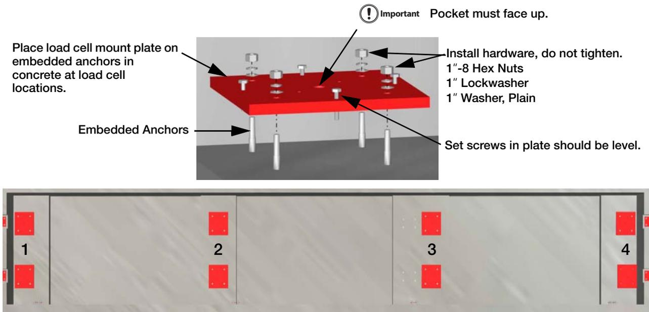
Top View of Load Cell Locations - 3 Module, 4 Section Scale Shown
