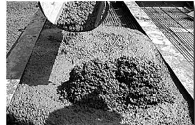
Position the unloading chute at the far side of the scale over the first bay. Begin filling the first bay, having the truck slowly move away from the scale to fill the bay uniformly.
