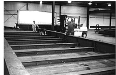
**Independent Modules:** If the next module is not to be bolted to the first, set the side rail 1" from the adjoining side rail. The final side rail will end 1.5" from the approach.
