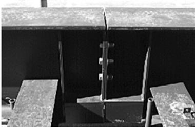
Set all side rails with the cut-outs for the load cell mount down and the uncut flange up. The headed anchor rods (Nelson studs) that will be encased in the concrete deck face inward.
