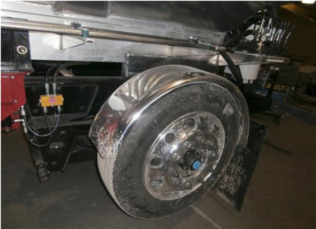
Figure 2-6. Support Spacer on an Aluminum Body
