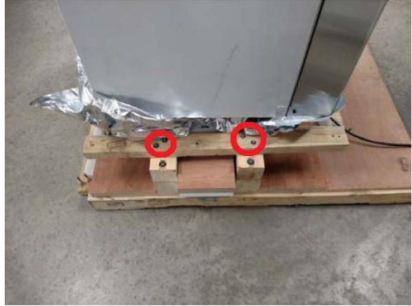
4.2 Remove the **four 17mm bolts** fastening the 4x4 braces spanning the width of the wrapper (left side of wrapper pictured, remove both sides):
