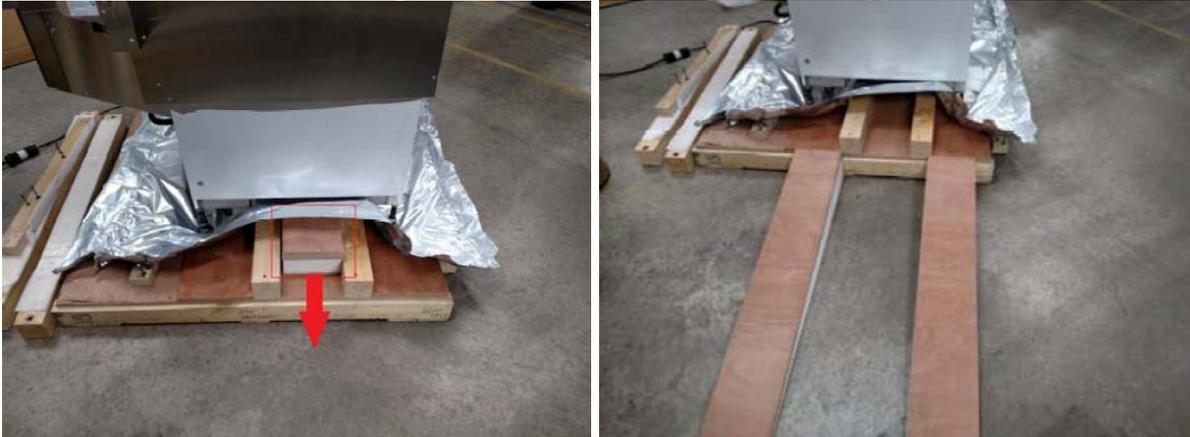
4.5 Raise all **four** leveling feet at even increments until the casters touch the pallet; continue raising the leveling feet counter clockwise until they cannot be raised any higher:
