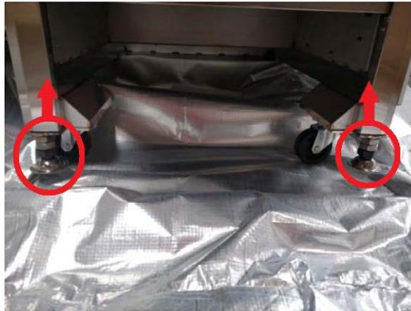
4.6 Roll the machine to the right, down the ramps and off the pallet as shown below; it's recommended to have **two** or **more** people guide the machine off the pallet.
