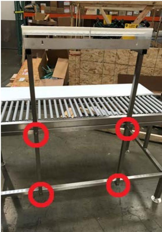
7.2 Install the dispenser for the small pop labels (**73065**) onto the pack-off table using supplied **four bolts/washers** for the vertical arms into the threaded pack-off frame, as seen to the left:
