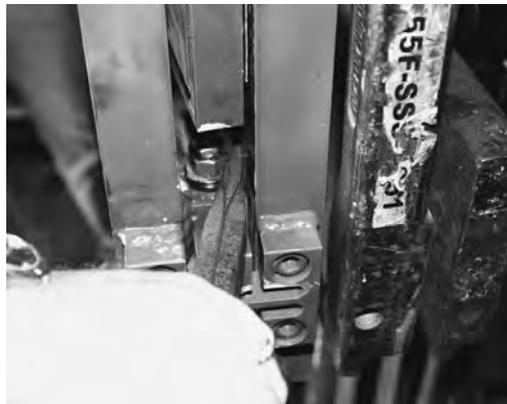
Figure 4-37. Center Load Cell
