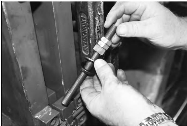
Figure 4-35. Install Spherical Washer Set
