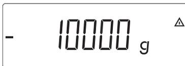
You will then be prompted to place the calibration/adjustment weight on the platform (e.g. 10 kg)
