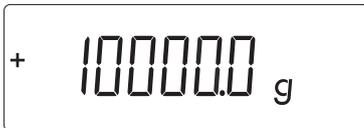
The calibration weight is displayed once calibration is finished.
