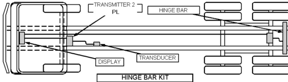
Figure 4-35. Block Diagram of Typical Hinge Bar Kit
