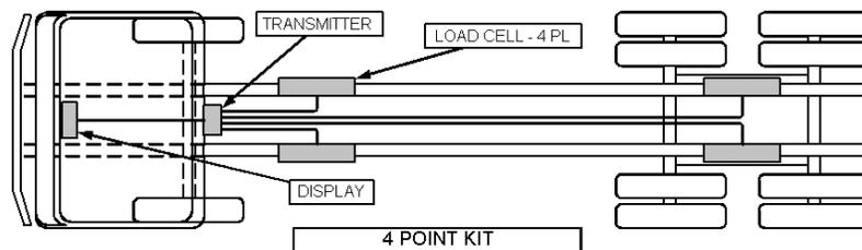
Figure 4-7. 4 Point Underbody Load Cell Kit
