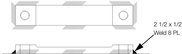
Figure 6-2. Weld Example of Single Piece Bearing Plate
