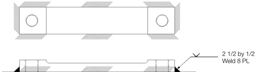
Figure 4-18. Bearing Plate
