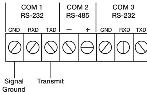
Figure 4-49. Model PL9710 Printer Connections
