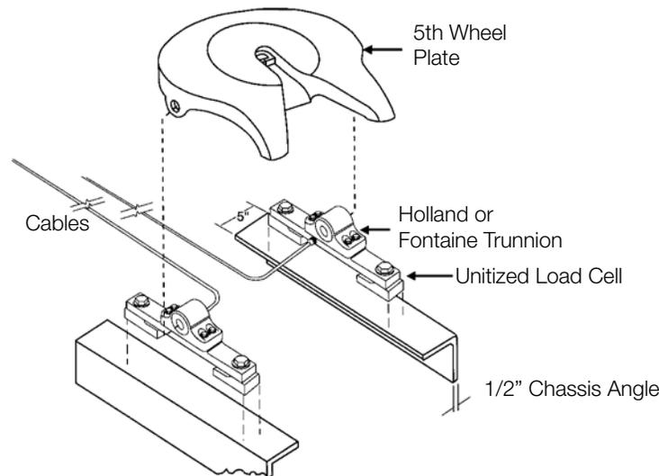
Figure 4-28. 5th Wheel Exploded View
