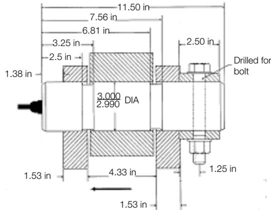
Figure 3-9. Typical Pin and Collar Assembly
