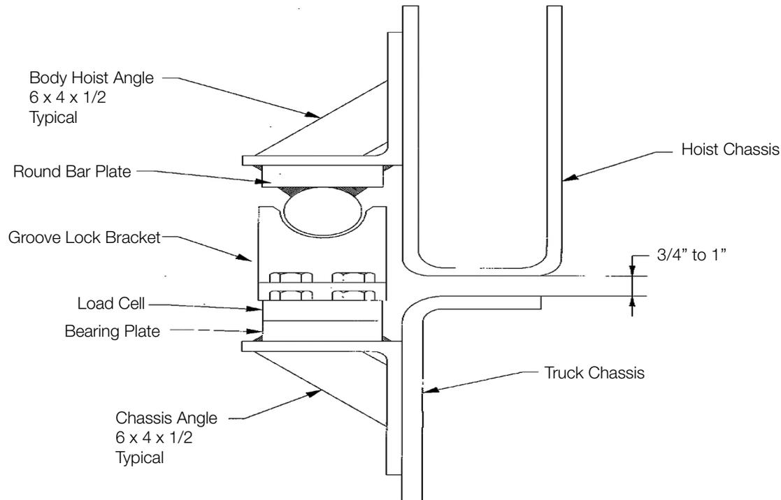
Figure 4-40. Groove Lock End View Showing PL9000-14 Load Cell
