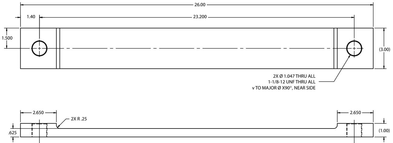
Figure 3-7. Optional Bearing Plate Specifications
