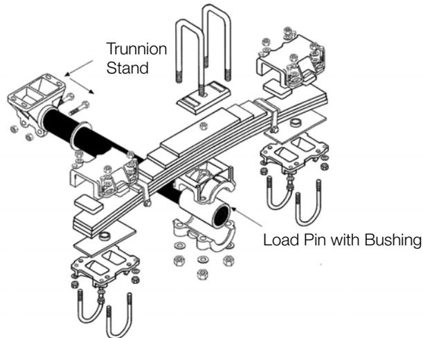
Figure 4-42. Exploded View of a Trunnion Installation
