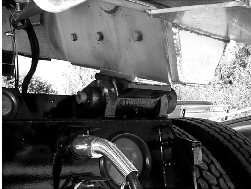
Figure 4-29. Hinge Pivot Installation
