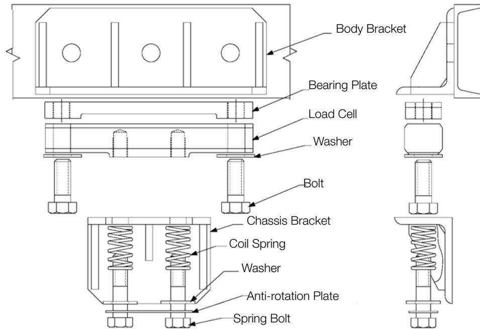
Figure 4-14. Mounting Springs, PL9000-14.4 Load Cell Installation
