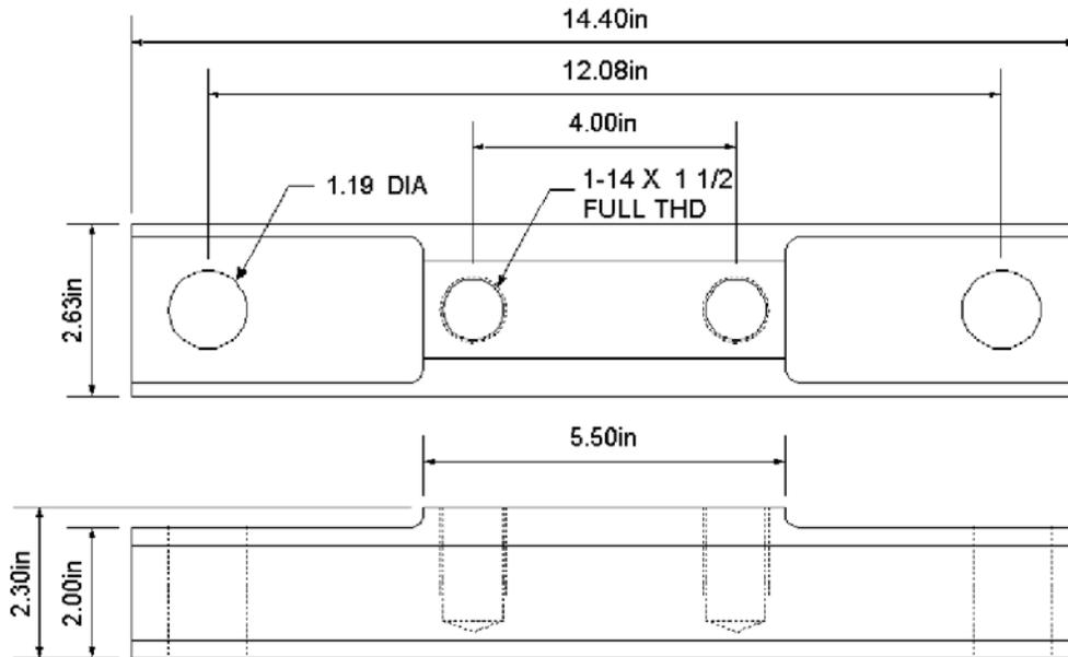
Figure 3-3. Model PL9000-14.4 Cell Specifications
