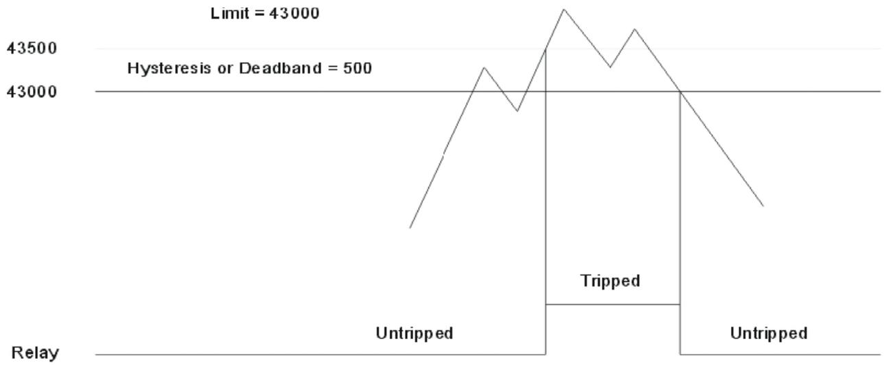
Figure 6-7. Typical Relay Limit Operation
