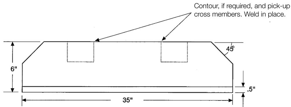
Figure 4-10. Extended Body Bracket for More Reinforcement
