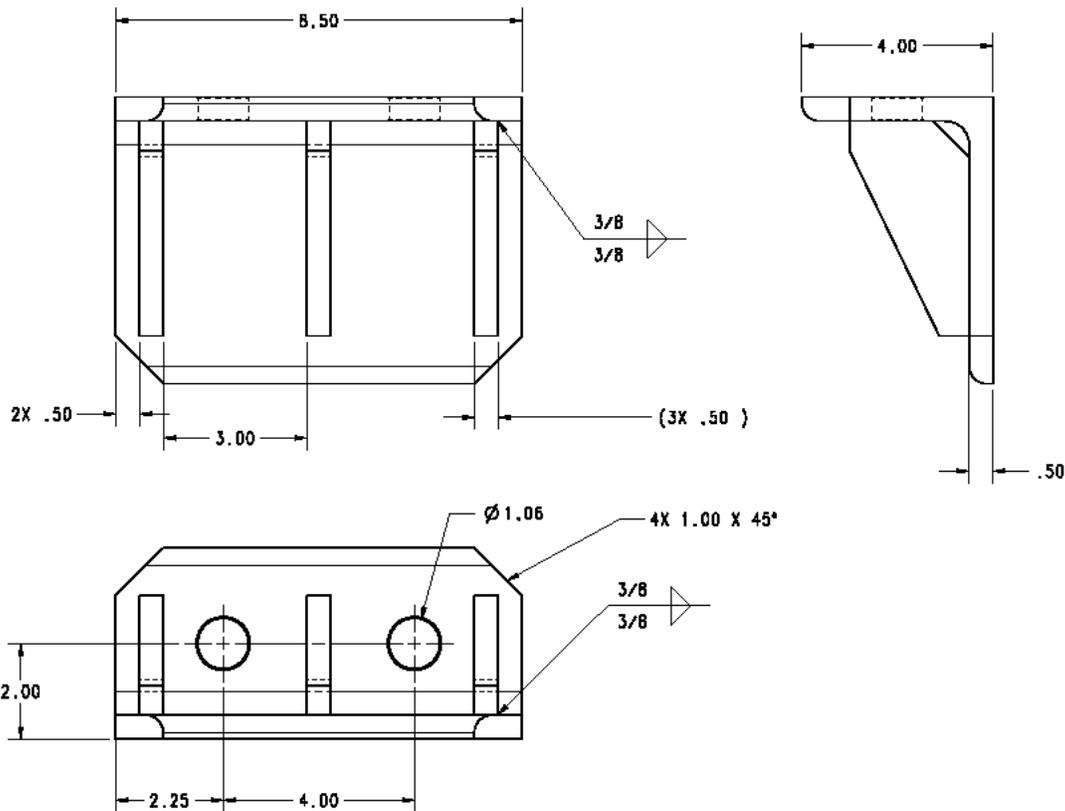
Figure 4-11. Chassis Bracket
