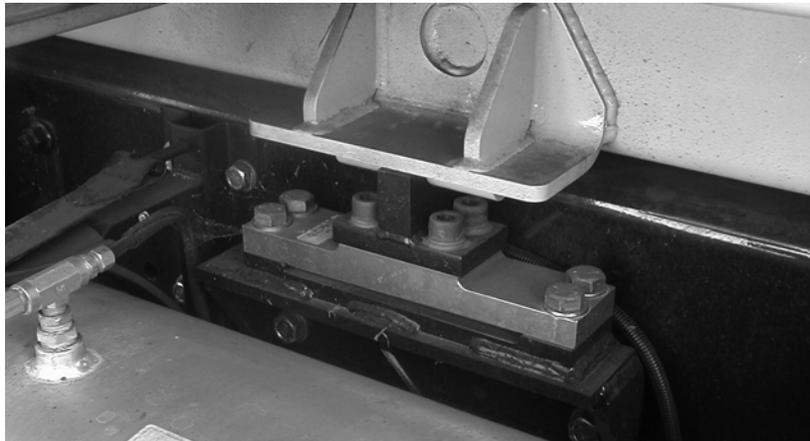
Figure 4-39. Body Rest Installation Example
