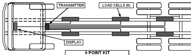
Figure 4-8. 6 Point Underbody Load Cell Kit
