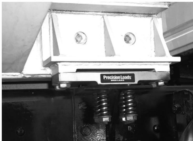
Figure 4-13. PL9000-14 Load Cell Coil Spring Mount Assembly
