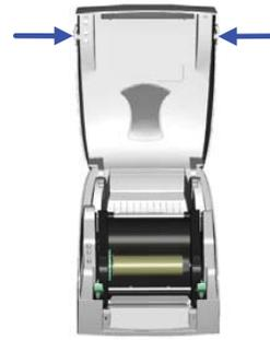
2. Place the label roll onto the label roll core.
