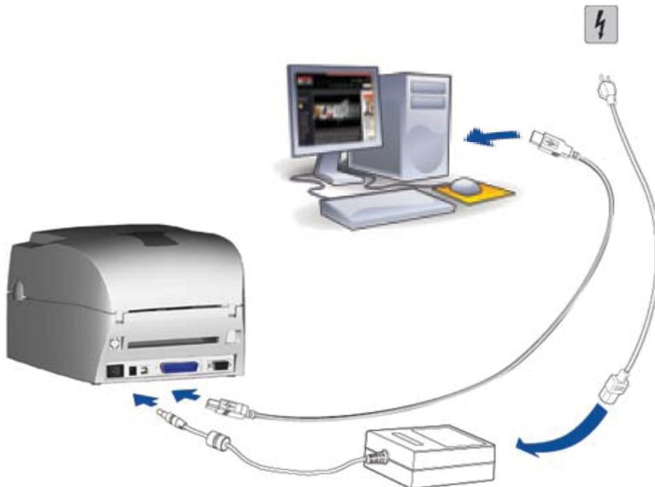
Figure 2-2. PC connection illustration
