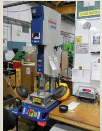
GTR Scales' solution guarantees the checkweighing step occurs before welding. If the weight of the set of filters does not fall into the allowable tolerance, or “accept band” of the CW-90, the sonic welder will not operate.
