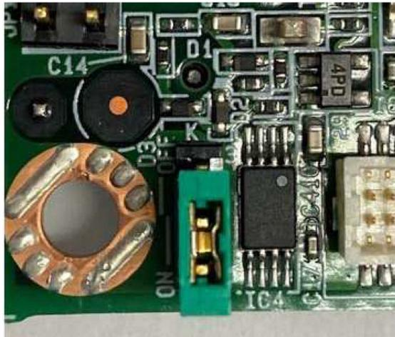
The battery jumper should be at the ON position (down) when viewed from the direction in the first photo.
